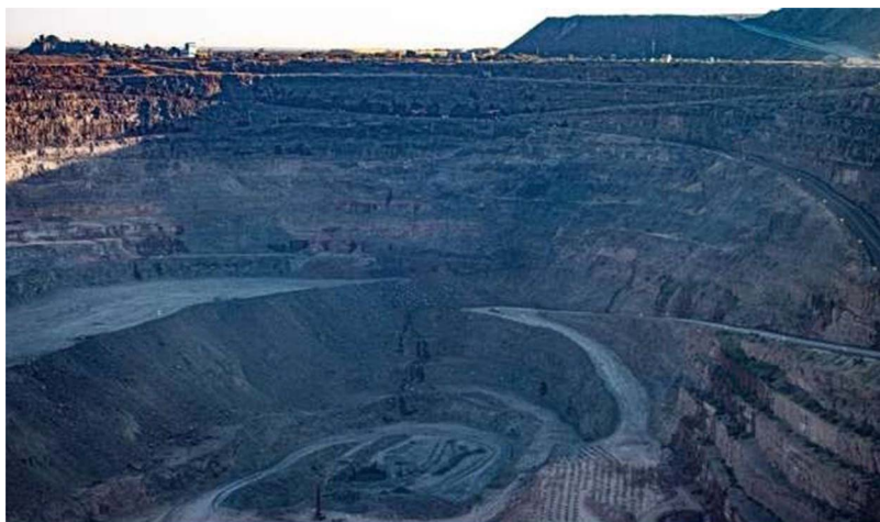
Fig. 1. Top view of the Orapa Diamond Mine showing the open pit left after the removal of the crater lake facies and kimberlite (21°18.465'S; 25°22.177'E). Photo by I.J. McKay, June 2018.
