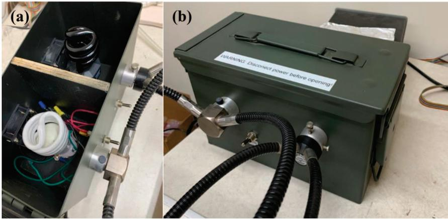
**Fig. 3.** Interior (a) and exterior (b) of dual light fixture used for *Pangaeus bilineatus* wavelength response bioassays.
