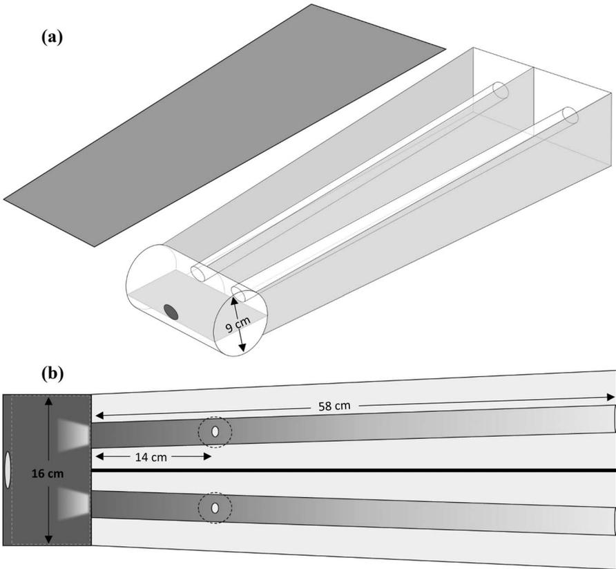
**Fig. 2.** Illustrations (not to scale) of test chamber used for *Pangaeus bilineatus* wavelength response bioassays: (a) oblique view of test chamber with lid and (b) overhead view of test chamber. Holes were drilled into the bottom of each treatment tube (14 cm from stage area) to trap peanut burrower bugs after they made a choice.
