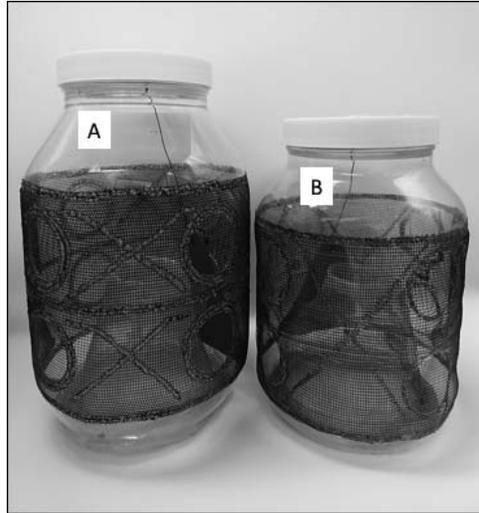
**Fig. 1. Two types of insect-collecting tops, namely, one using a 3.8-L jar (A) and other with a 2.8-L jar (B), for stink bug pyramid traps.**
