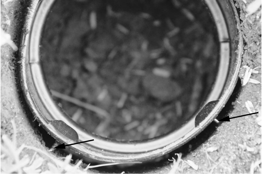
Fig. 2. Overhead view of collar, showing nails used to anchor it in hole (arrows).
