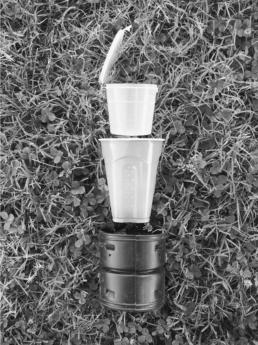
Fig. 1. Components of the pitfall trap (top to bottom): reservoir, liner, collar.
