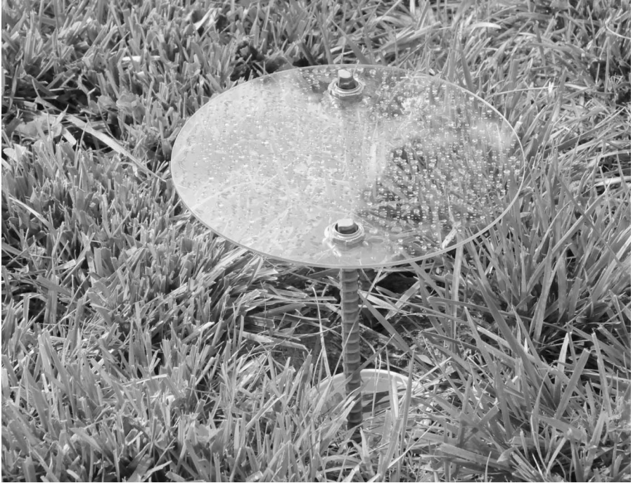
Fig. 4. Oblique view of trapping station, showing deployment of polycarbonate cover, festooned with droplets from a recent rainfall.
