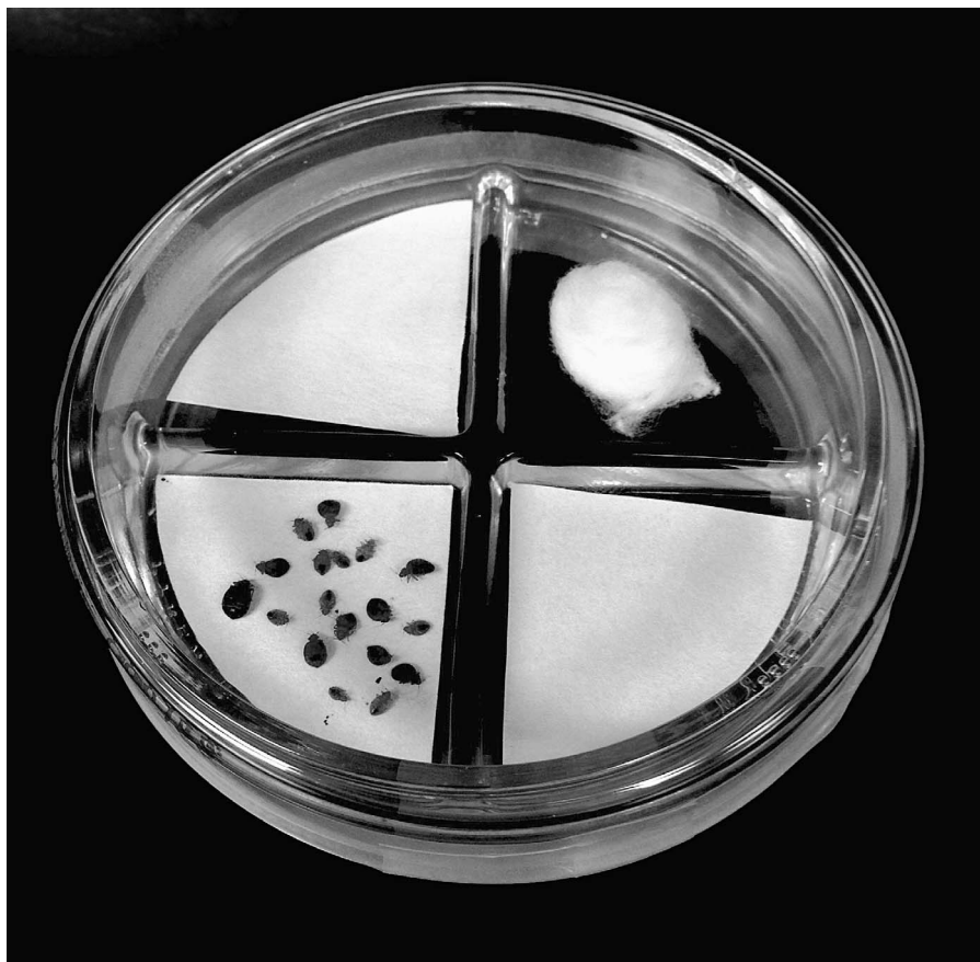
Fig. 1. Petri dish experiments. Mock-up showing divided Petri dish used for initial screening of compounds for fumigation activity. Bed bugs were placed in one quadrant of the dish and test compounds were applied to cotton ball. The Petri dish was then sealed with parafilm. Mortality was assessed 5 d posttreatment.
