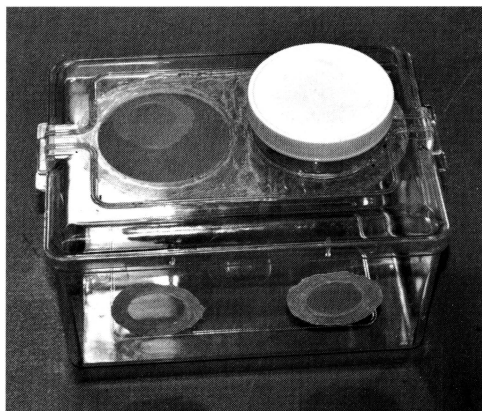
Fig. 2. Smaller version of the rearing cage design. The bottom has only 6 windows, two in each of the larger sides and on in each of the shorter sides. The tom of the cage has only one aeration window and one water niche and no access opening. All windows had the same dimensions as in the larger cage version.
