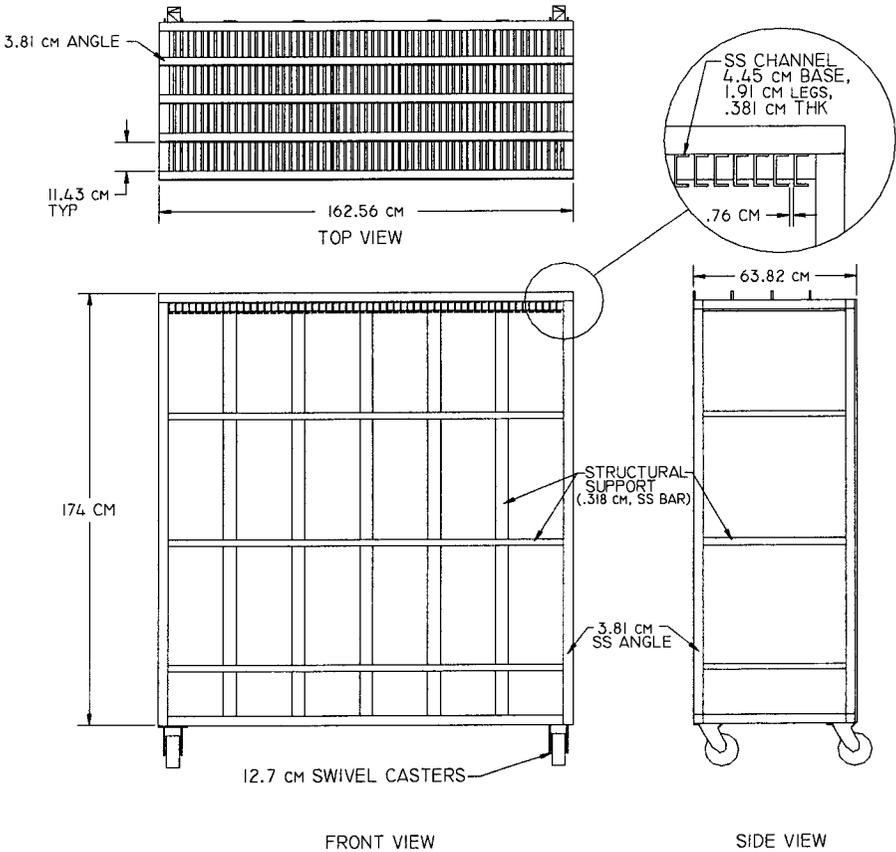
Fig. 3. Specifications for a new full-sized cart with a capacity of 1296 rearing trays.
