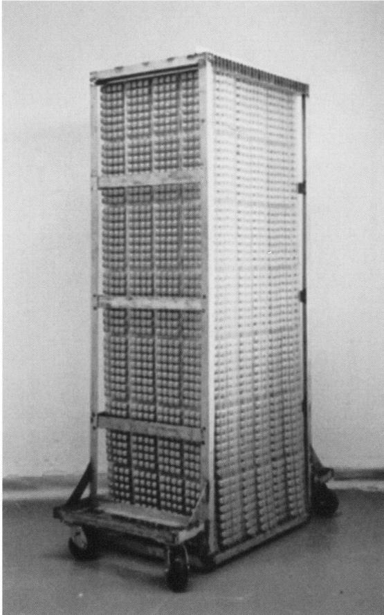
Fig. 2. View of the half-width test model of the new cart filled with 7-tray cuts.
